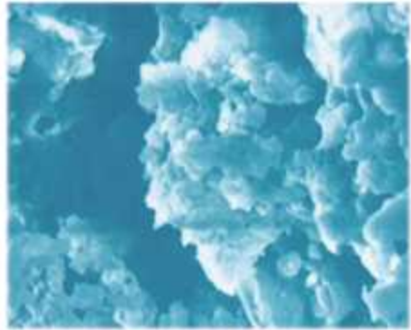
Untreated concrete (enlarged 4000 times)
